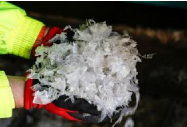
Photo 3: Shredded plastic after the Vecoplan shredder
